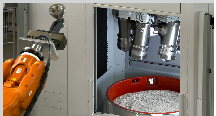
Robot attaching a work piece to a workstation in the drag finisher
