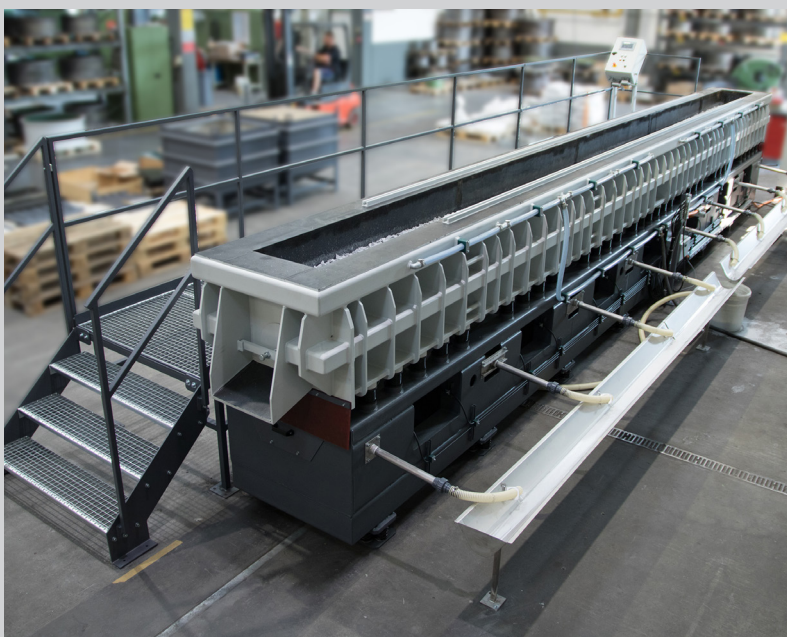
Extra long tub: Length of processing channel = 7,400 mm (25 ft.)
