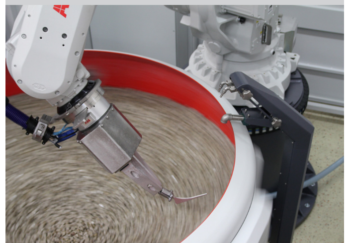
Glimpse into the rotating work bowl: Robot-guided work piece
